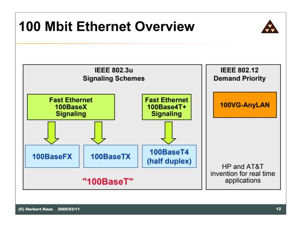
The diagram above gives an overview of 100 Mbit/s Ethernet technologies, which are differentiated into IEEE 802.3u and IEEE 802.12 standards. The IEEE 802.3u defines the widely used Fast Ethernet variants, most importantly those utilizing the 100BaseX signaling scheme. The 100BaseX signaling consists of several details, but basically it utilizes 4B5B block coding over only two pairs of regular Cat 5 twisted pair cables or two strand 50/125 or 62.5/125-µm multimode fiber-optic cables.
